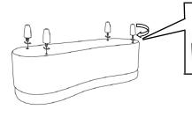
Remove the plastic caps from screw heads before attaching legs.
