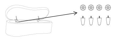
Step 2.Screw legs into pre-drilled holes until tight.
